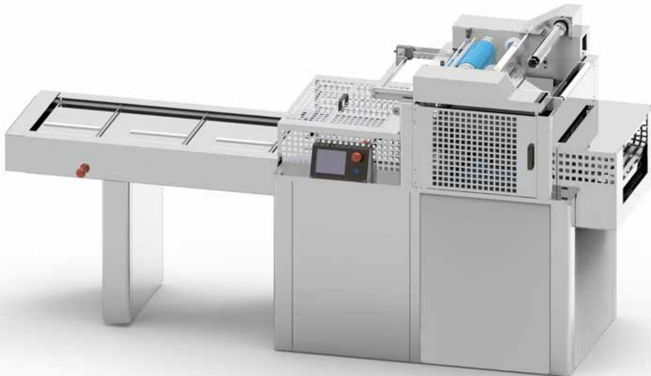
The line of thermo sealers Silvy is designed for the automatic packaging of preformed trays with compatible closing film. The machine Silvy is available in two different models. The complete version allows the realization of trays in 4 different technologies: only sealing, ATM, vacuum or skin. The simplified version, Silvy N, is ideal if you only need to seal.
